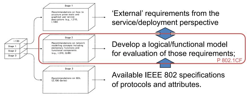
• A 'Stage 2' specification would provide a mapping of the existing IEEE 802 protocols to a functional network model, which facilitates easier evaluation and better understanding of end-to-end behavior.
