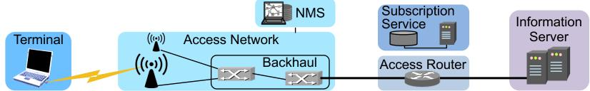
The portion of the access infrastructure in scope of IEEE 802 was defined according to the protocol layer architecture of the data path
