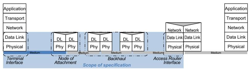
IEEE 802 access network describes the layer 2 network between terminal and access router implemented through IEEE 802 technologies.
