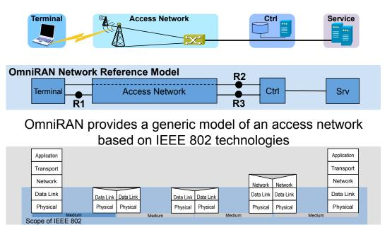
Fig. 2: Access Network Abstraction, per omniran-13-0048-04-ecsg, etc.
