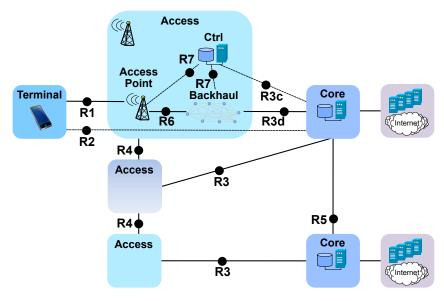
Fig. 8: Network Reference Model with Backhaul, with dotted lines representing controlonly links
