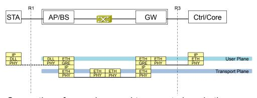
Separation of user plane and transport plane in the access network leads to the definition of a 'backhaul'
