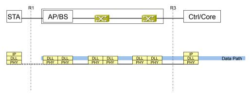
OmniRAN defines an access network without separation of user plane and transport plane in isolated networking layers. Backhaul can be considered integrated into the data path in OmniRAN.
