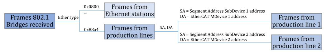
All the SubDevices of the segment will not change the destination MAC address of the EtherCAT frame, and the EtherCAT frames will be forwarded to next specific SubDevice other than according the destination MAC address.
