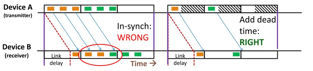
Annex T of IEEE 802.1Q-2018 fixes long link delay by adding dead time, which reduces the bandwidth available for CQF streams and sets a minimum cycle time.
