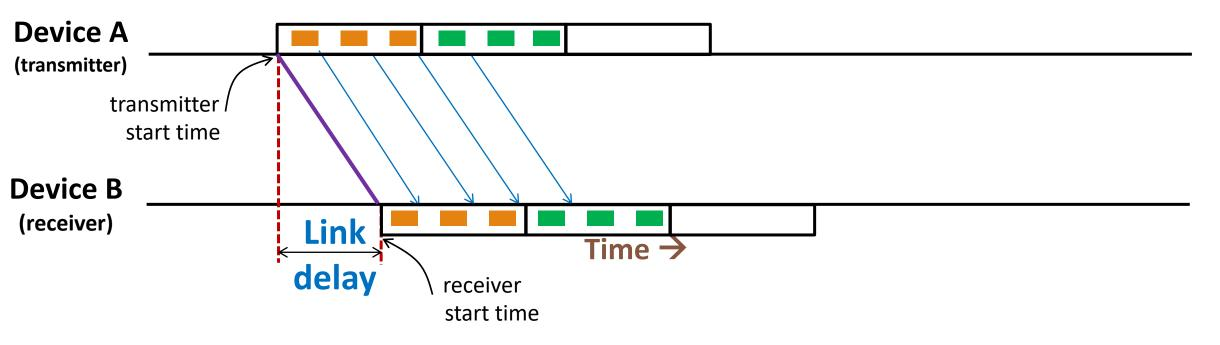
• We want offset the cycle start time of the receiving input gates from the transmitting output gates by an amount equal to the link delay.
