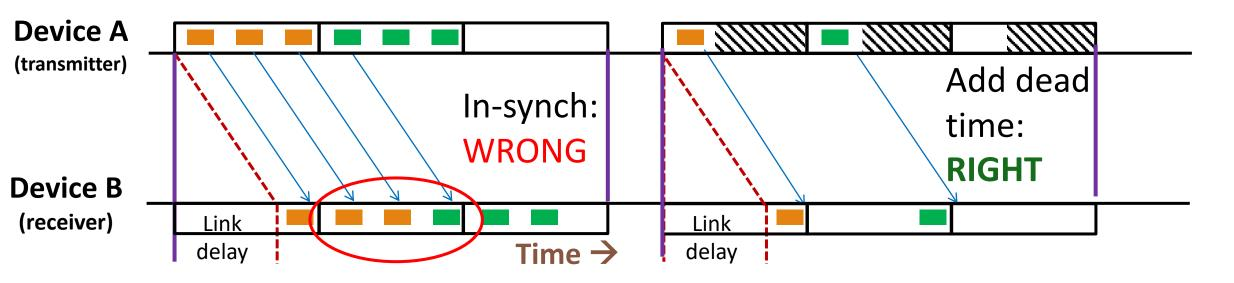
Annex T of IEEE 802.1Q-2018 fixes long link delay by adding dead time, which reduces the bandwidth available for CQF streams and sets a minimum cycle time.
