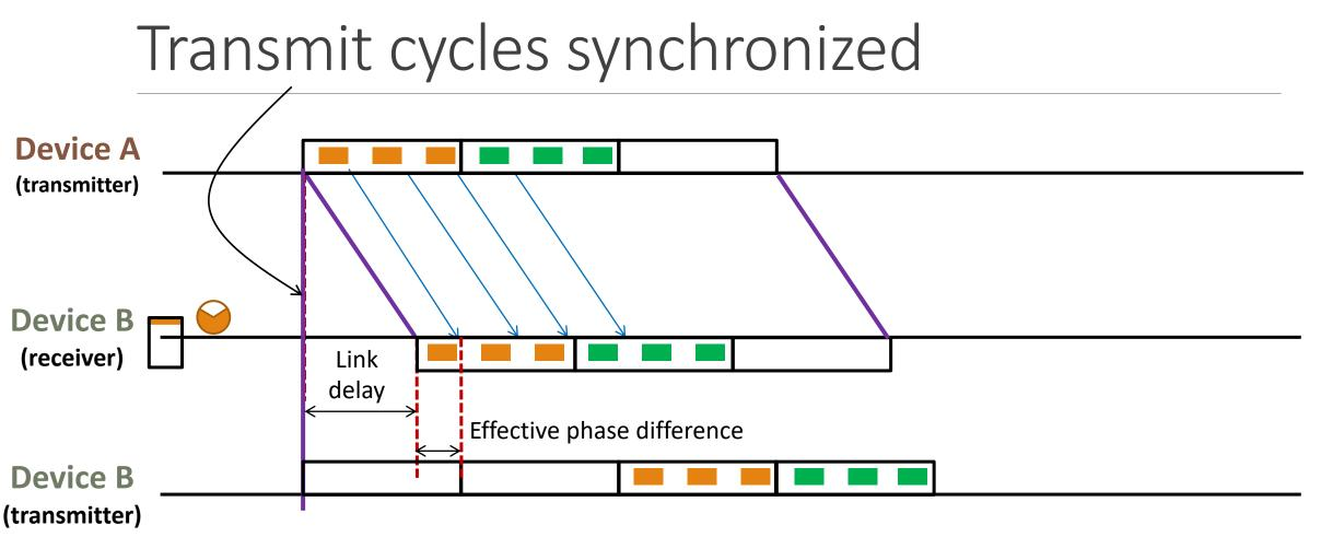
• The "effective phase difference" determines the CQF buffering delay in device B. If it is small, two buffers and a little dead time can be used.
