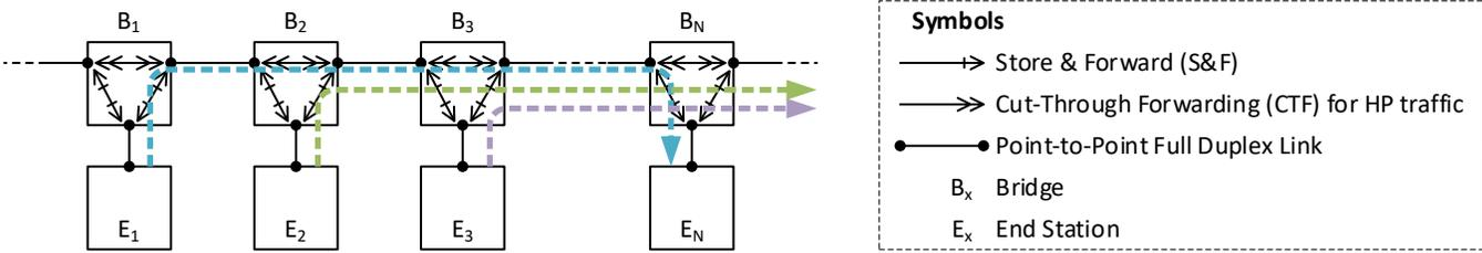
Delay until forwarding to destination port(s). Assumed that the lookup starts after  $l_{Hdr}$  octets and finishes after  $d_{LU}$   $\mu s$ . Note that the lookup can finish after frame completion during reception.
