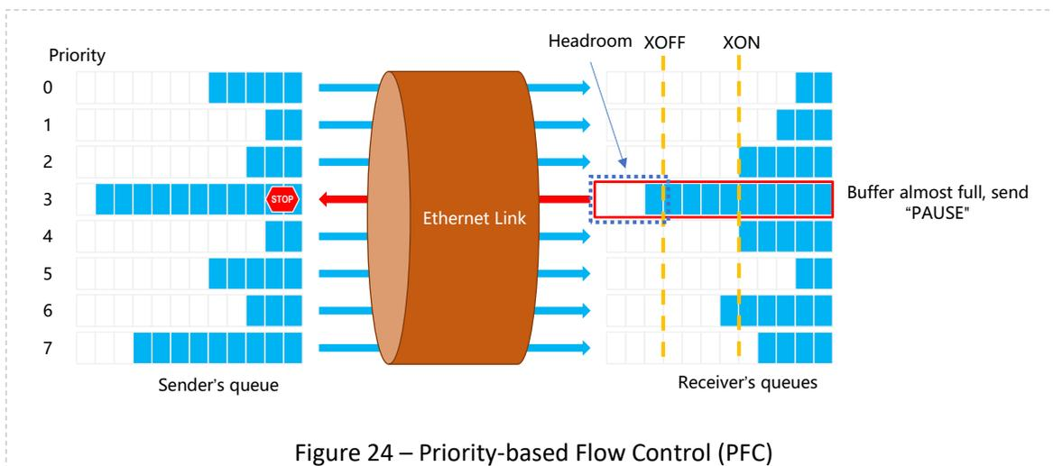
Figure 24 – Priority-based Flow Control (PFC)
