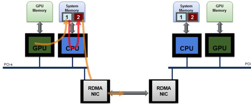
**Figure 14: The Data Transfer Before GPU DirectRDMA**
