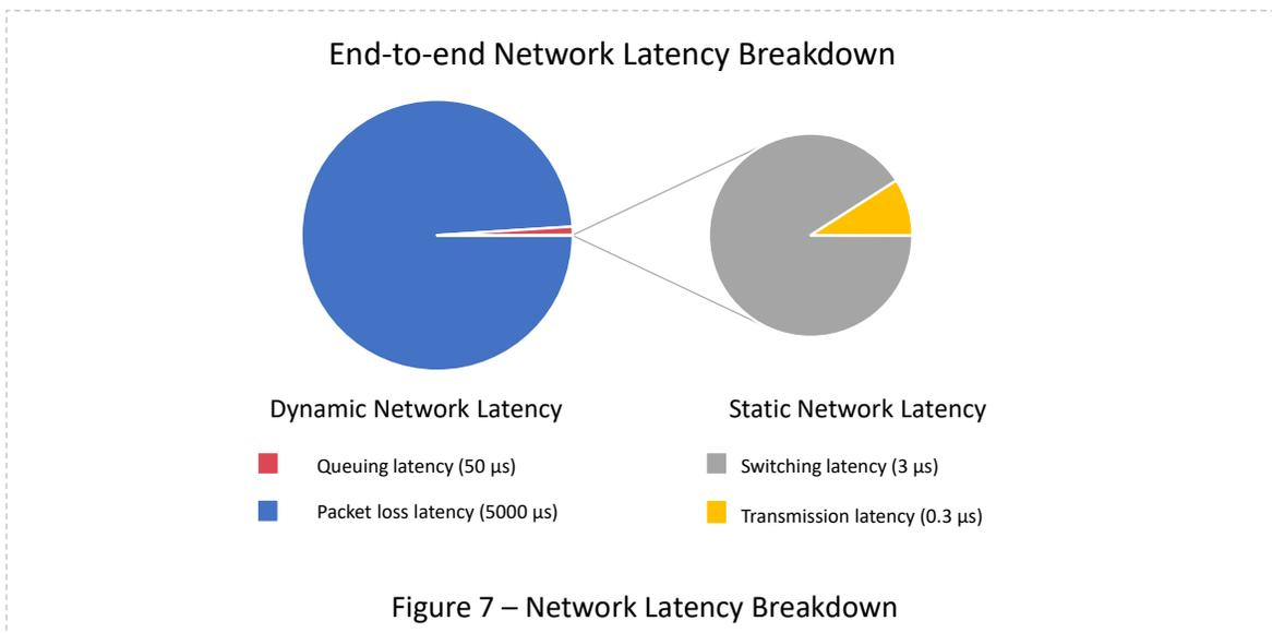
Figure 7 – Network Latency Breakdown
