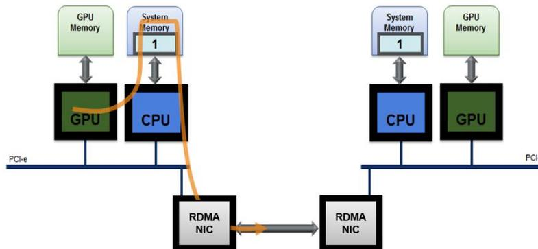
**Picture 15: The Data Transfer Using GPU Direct**
