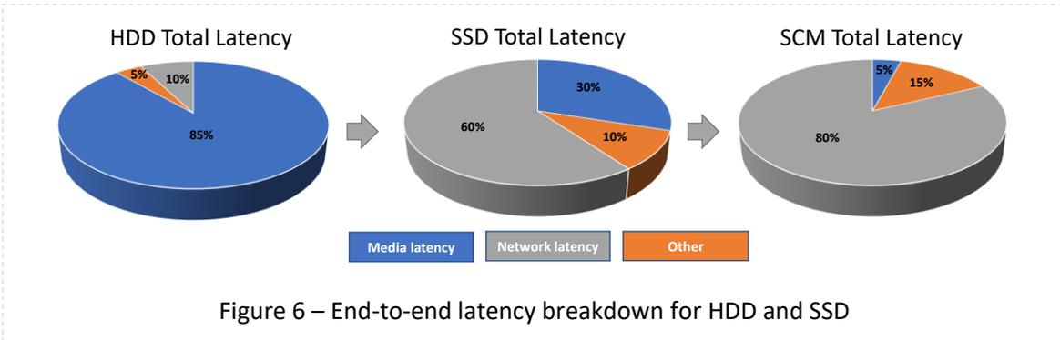
Figure 6 – End-to-end latency breakdown for HDD and SSD
