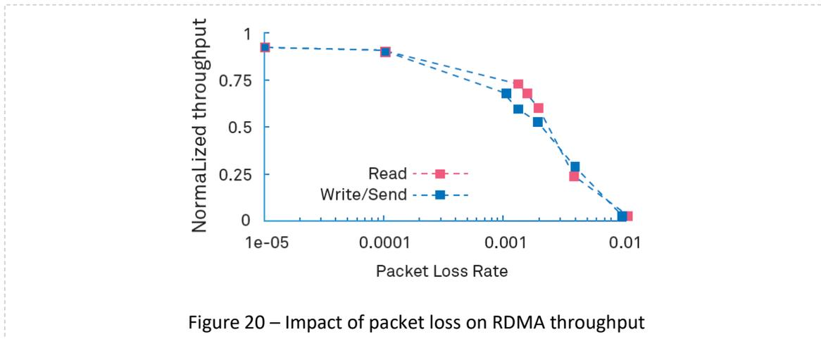
Figure 20 – Impact of packet loss on RDMA throughput
