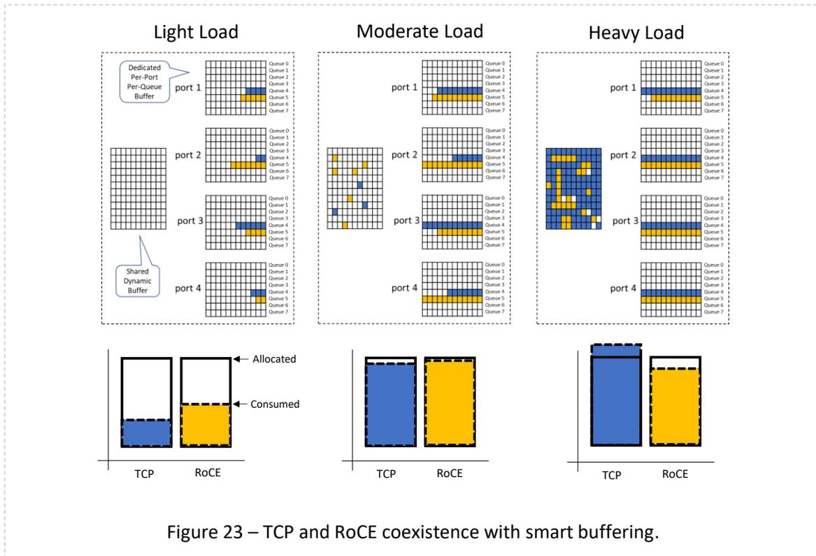
A core idea of smart buffering is the creation of a dynamic shared buffer. The goal is to optimize buffer utilization and burst absorption by reducing the amount of statically dedicated buffers while providing a dynamic and self-tuning shared pool across all ports to handle temporary bursts [25].
