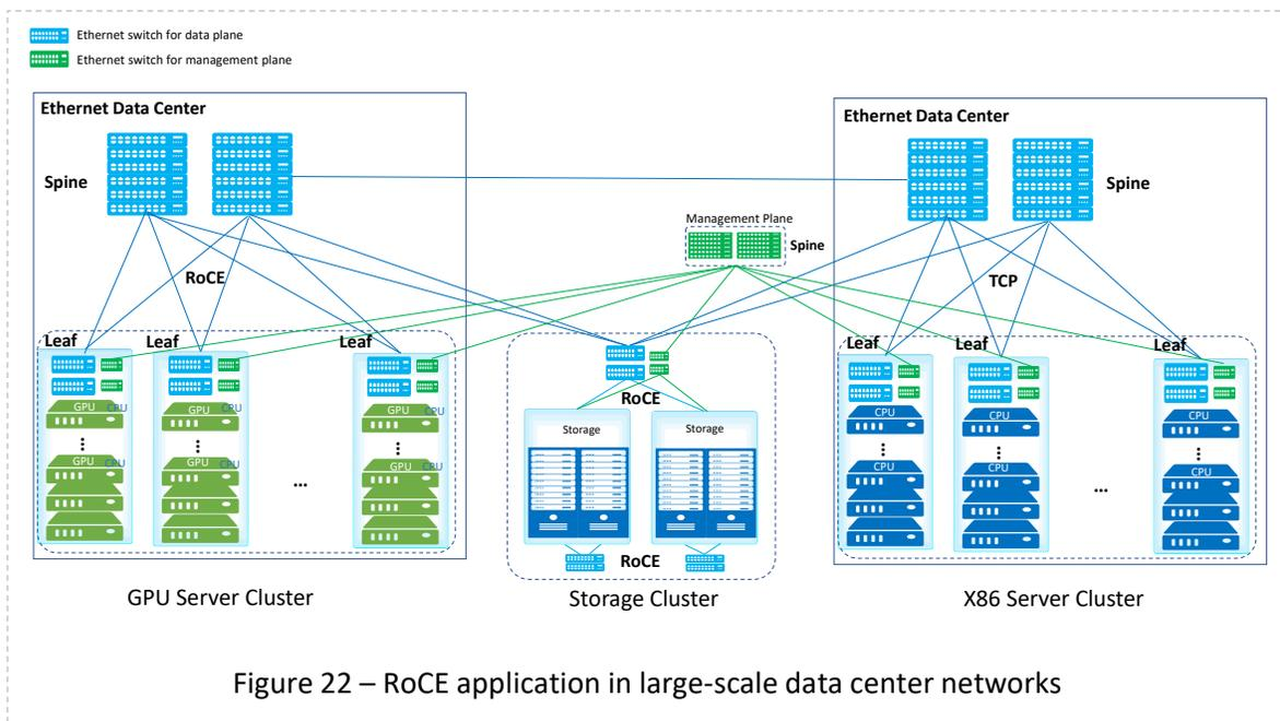
Figure 22 – RoCE application in large-scale data center networks
