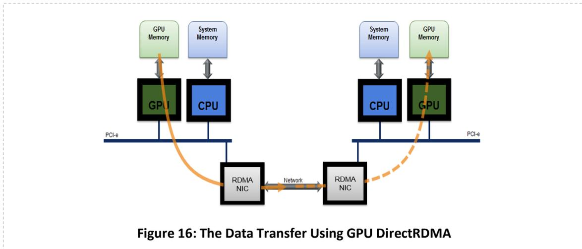
**Figure 16: The Data Transfer Using GPU DirectRDMA**
