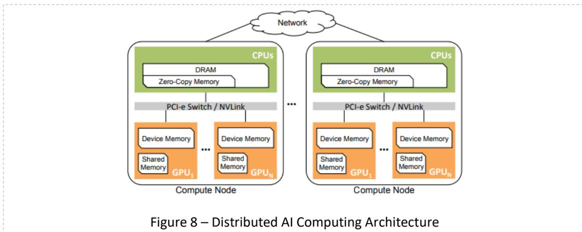
Figure 8 – Distributed AI Computing Architecture
