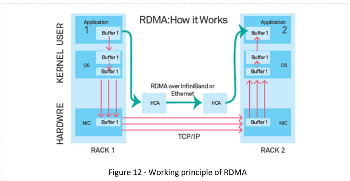
There are three different transports for the RDMA protocol: Infiniband, iWarp and RoCEv1/RoCEv2.
