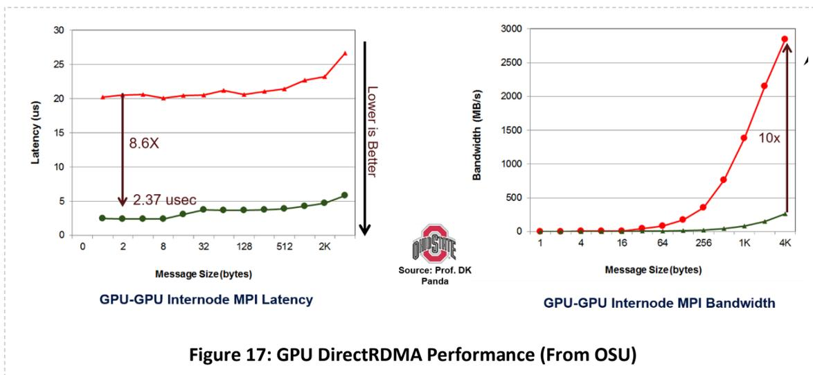
**Figure 17: GPU DirectRDMA Performance (From OSU)**
