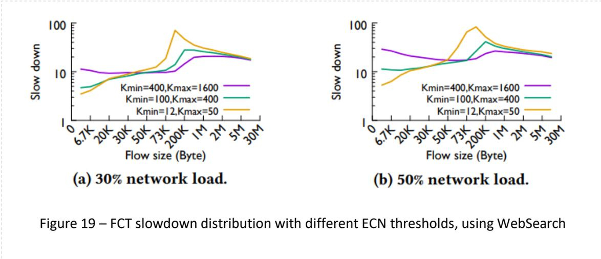
Figure 19 – FCT slowdown distribution with different ECN thresholds, using WebSearch
