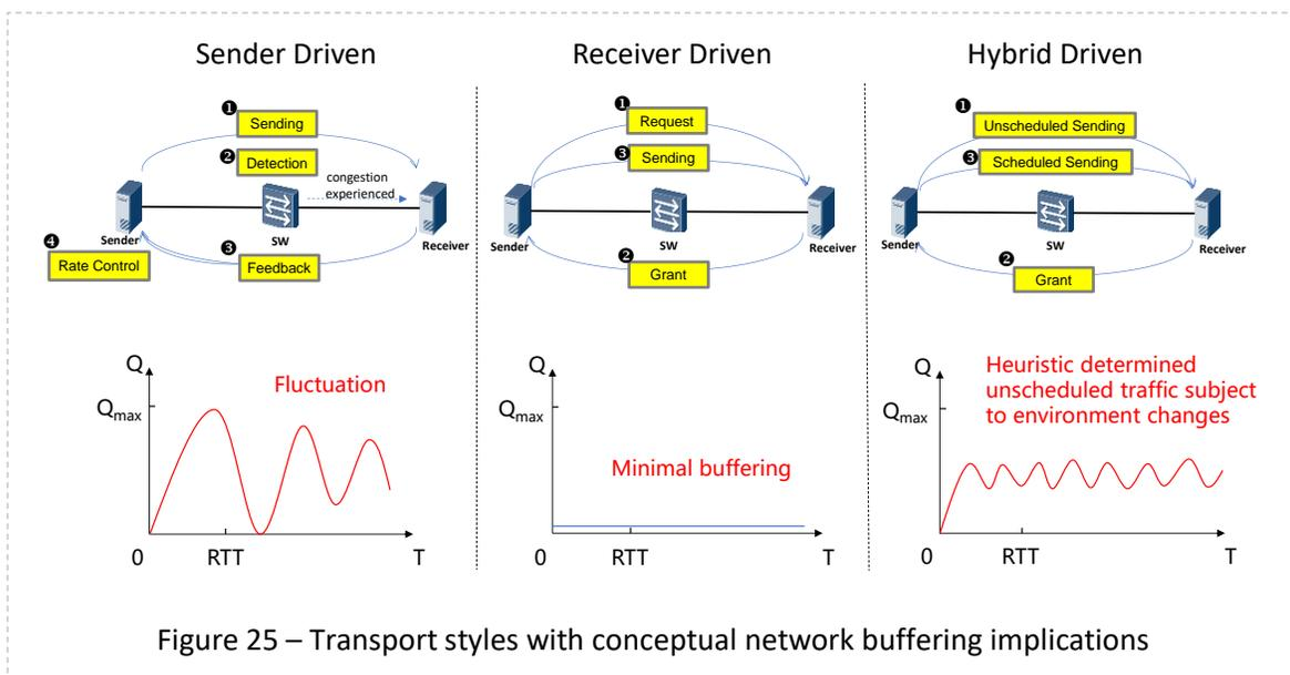
those congestion signals first. Perhaps a more significant challenge with receiver driven transports is the inherent delay built into the initial buffer request by the sender. The initial request-grant exchange penalizes small flows which, in most cases, are latency sensitive and constitute the majority of flows in the data center network.
