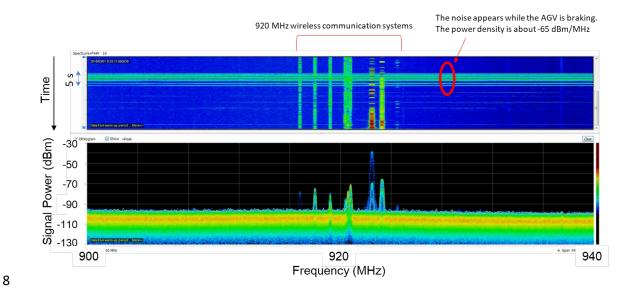
Figure 5—Measured noise spectral density
