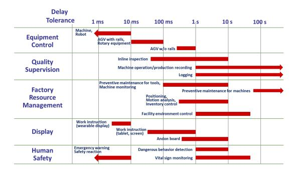
Figure 9—Permissible delay of representative wireless applications
