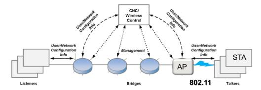
Figure 15—Centralized configuration heterogeneous network
