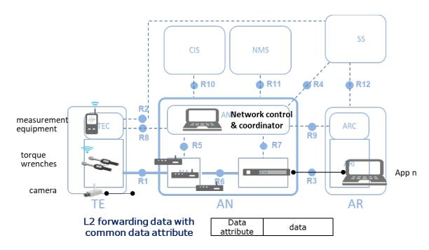
Figure 21—Mapping factory network to IEEE 802.1CF NRM
