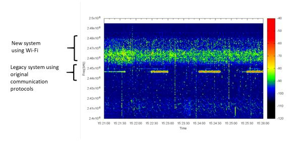
Figure 6—Wireless signals with coexistence of different wireless technologies—The vertical and horizontal-axes show frequency (Hz) and time, and color shows signal strength (dBm) in a bar on the right hand side
