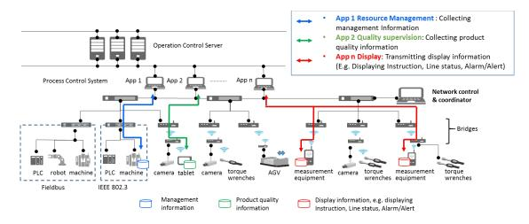
Figure 7—Wireless applications in factory
