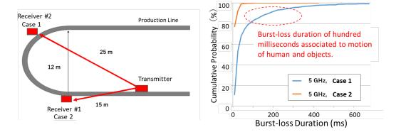
Figure 16—Burst-loss measurement in a large machine assembly site [26]
