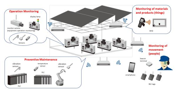
Figure 10—Usage scene: Metal working site
