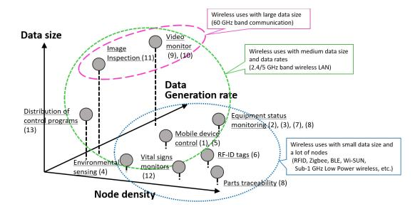
Figure 8—Representative wireless applications with corresponding classifications (1)–(13) from Table 1 and their wireless communication features
