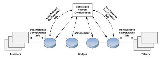
Figure 14—Centralized configuration bridge network
