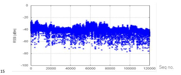
Figure 4—RSSI fluctuation in factory
