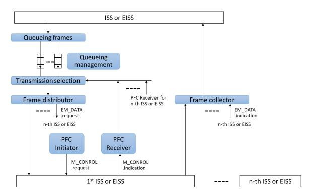
Figure 17—PFC aware system queue functions with Link Aggregation (Rewritten Figure 36-4 in IEEE Std 802.1Q-2018)
