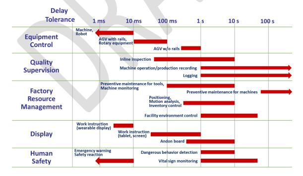
Figure 9 Permissible delay of representative wireless applications
