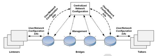
Figure 14 Centralized configuration bridge network
