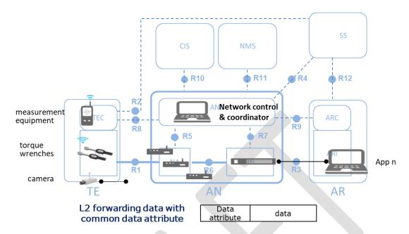
Figure 21 mapping factory network to 802.1CF NRM
