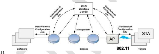
Figure 15 Centralized configuration heterogeneous network
