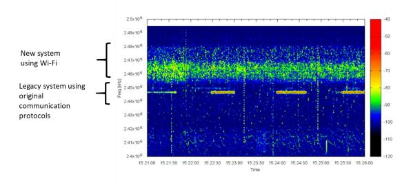
Figure 6 Wireless signals with coexistence of different wireless technologies. The vertical and horizontal-axes show frequency (Hz) and time, and color shows signal strength (dBm) in a bar on the right hand side.
