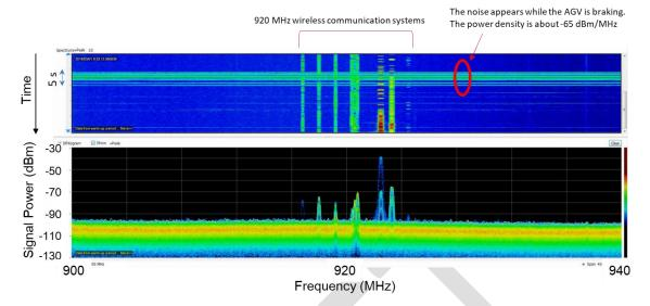
Figure 5 Measured noise spectral density
