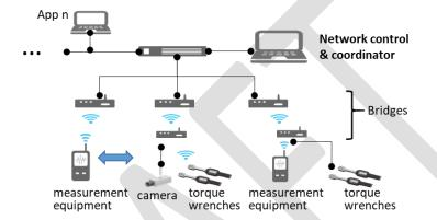
Figure 19 typical network scenario for flexible factory IoT
