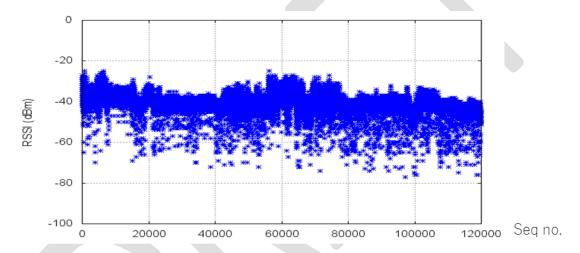
Figure 4 RSSI Fluctuation in Factory
