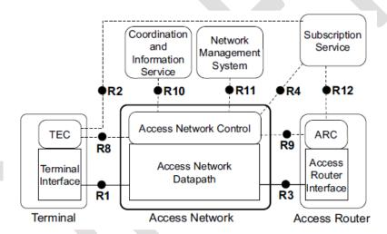
Figure 20 network reference model defined in IEEE P802.1CF
